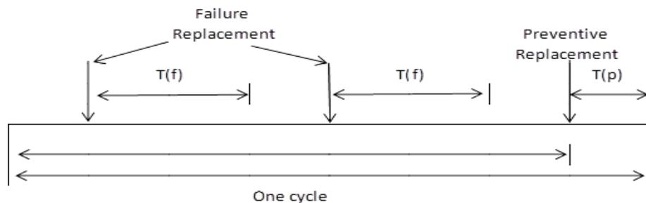
Figure 2: Downtime minimization: optimal interval.
